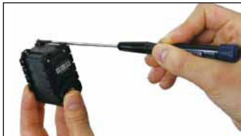
(1) Convenient AX-12+/AX-18F nut insertion method
